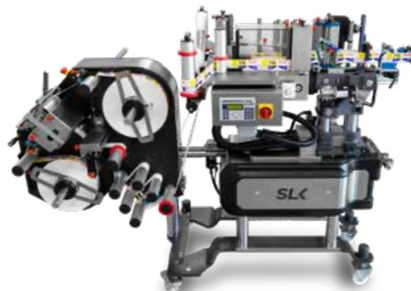
Pressure sensitive labeling station with automatic junction system.
