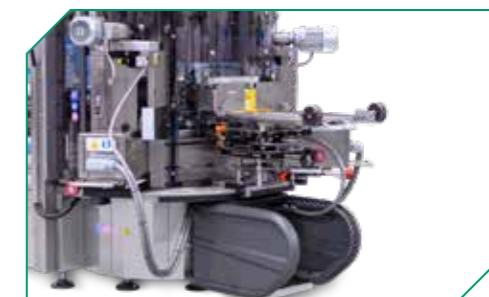
Hot melt labeling station for paper wrap-around applications.
