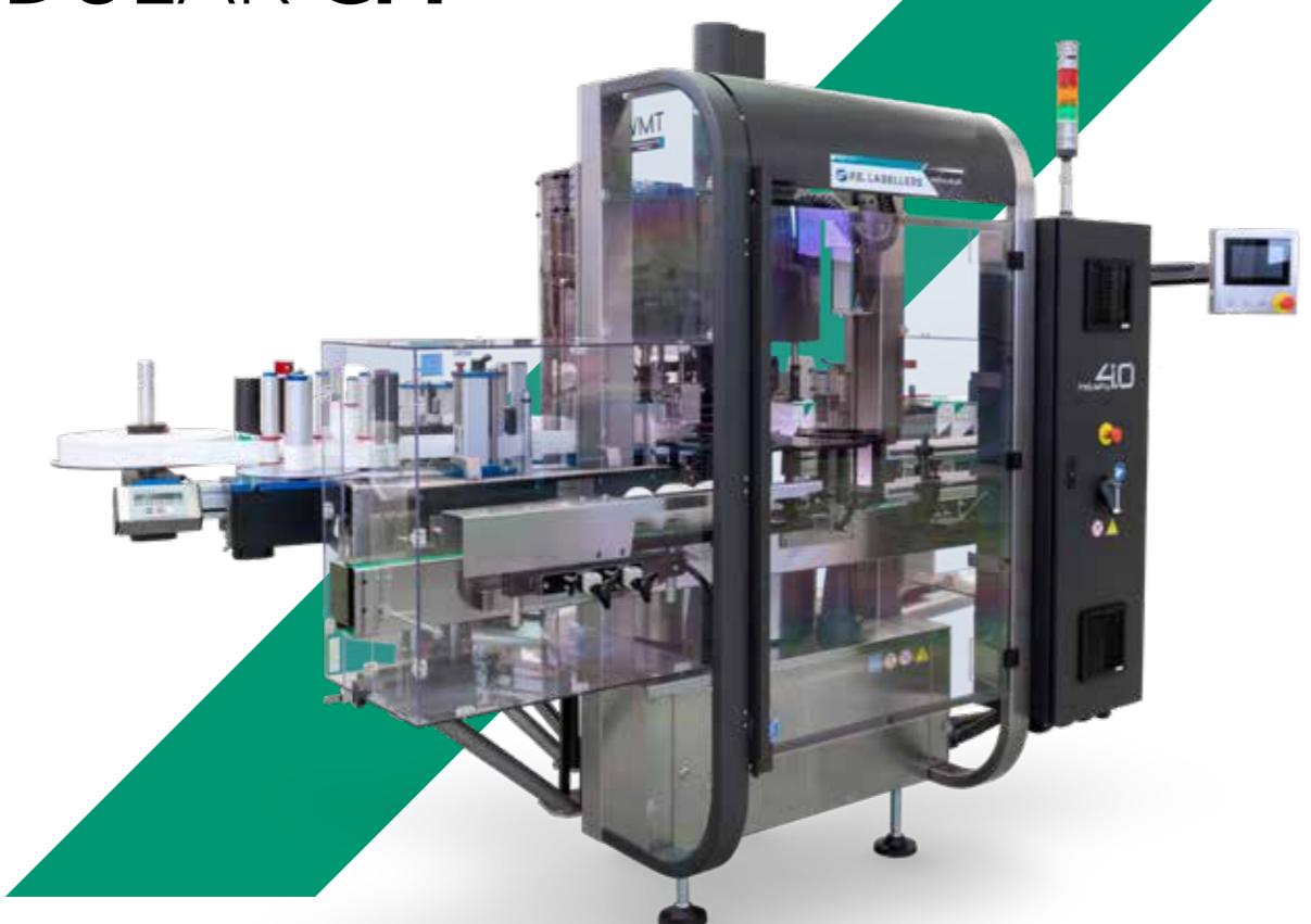
Modular CM is a completely ergonomic and modular automatic labeling machine with a layout that can be reconfigured quickly and easily.
