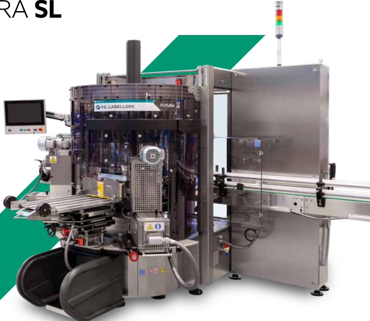
Futura SL is a solution with hot melt technology for the application of pre-cut wrap-around labels.
