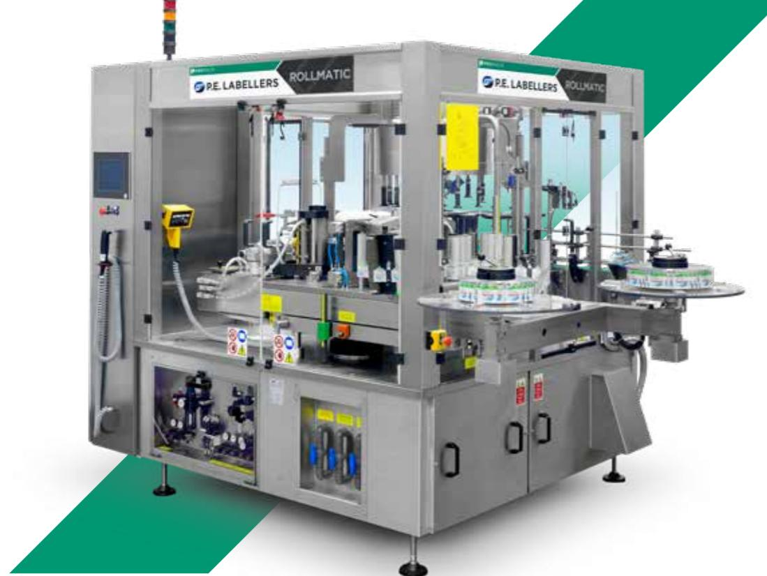
Rollmatic is a roll-fed rotary labeler for the application of wrap-around labels with hot melt. It can reach 60,000 bph and is available in four sizes.
