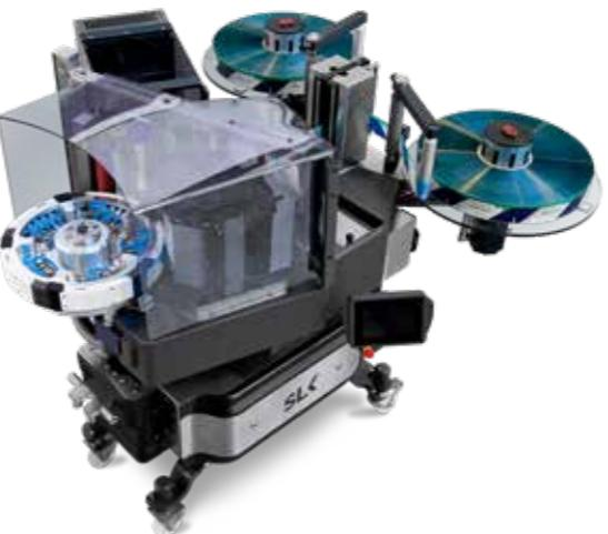
Simpl-Cut™ unit installed on cart (SLK) to be combined with a Modular SL machine.
