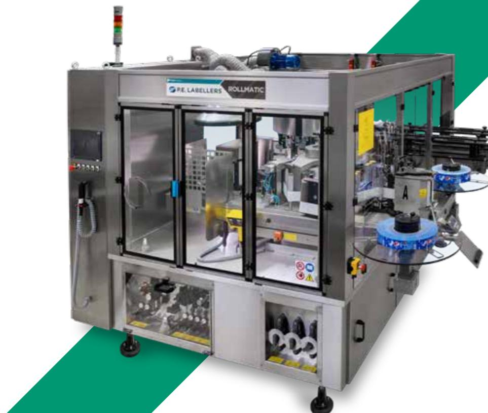
Rollmatic is a roll-fed rotary labeler for the application of wrap-around labels with hot melt. It can reach 60,000 bph and is available in four sizes.
