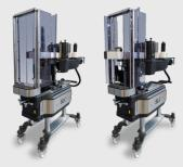
For pressure sensitive labelling station we designed "saloon doors" to prevent the access at the carousel when the unit is not in production.
