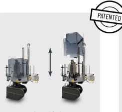
We equip the cold glue labelling units with up and down system that guarantee an easy access to the station for a quick change over.
