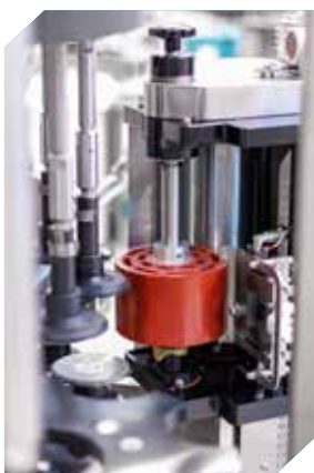
Roller for glue application on the container.
