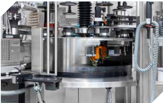
Machine with plate rotation by means of servomotors (optional).
