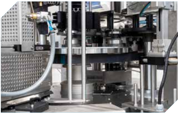
Machine with plate rotation by toothed belt (standard).
